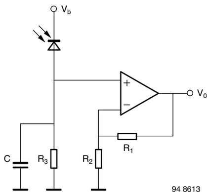
Fig. 23 - RC-Loaded Photodiode with Voltage Amplifier
