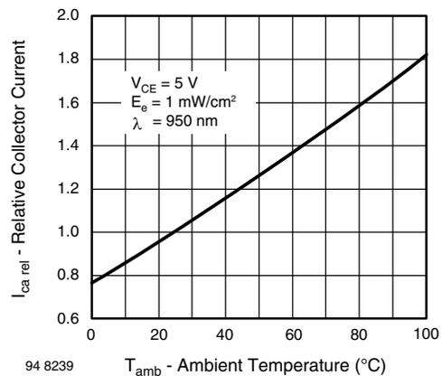
Fig. 2 - Relative Collector Current vs. Ambient Temperature
