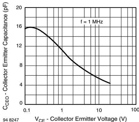
Fig. 5 - Collector Emitter Capacitance vs. Collector Emitter Voltage
