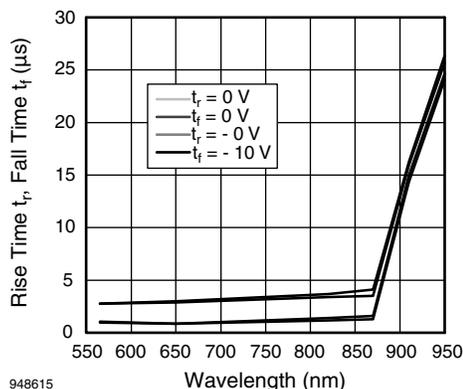
Fig. 25 - Switching Times vs. Wavelength for Photodiode BPW20RF
