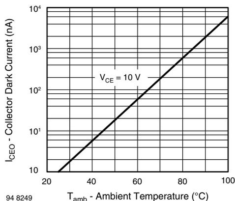
Fig. 1 - Collector Dark Current vs. Ambient Temperature
