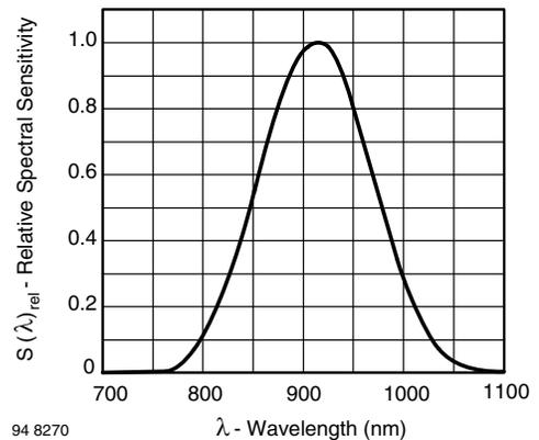
Fig. 7 - Relative Spectral Sensitivity vs. Wavelength
