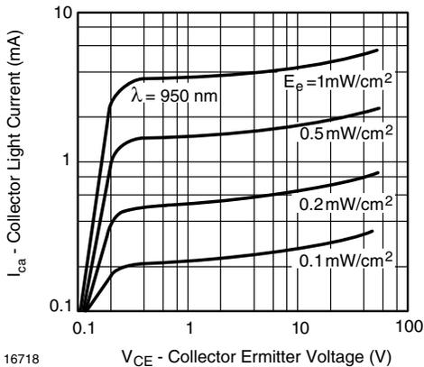
Fig. 4 - Collector Light Current vs. Collector Emitter Voltage
