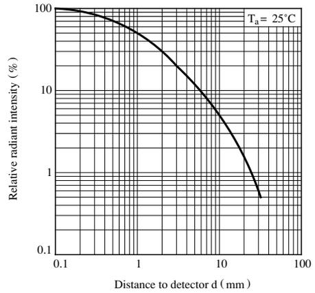
Fig. 9 Relative Collector Current vs. Distance (Detector : PT4800)
