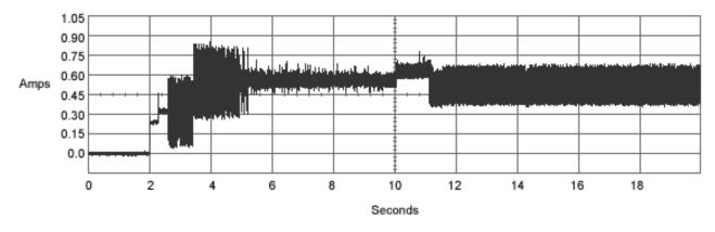
Figure 1. Typical 5V startup and operation current profile
