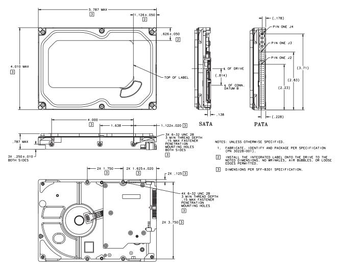
Figure 6. Drive dimensions for 40-160 GB and STM3250310AS models
