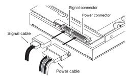
Figure 4. Attaching SATA cabling
