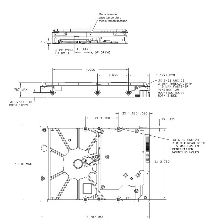
Figure 4. Mounting dimensions (500, 320, 250 and 160 GB models)
