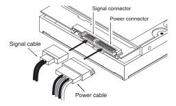
Figure 2. Attaching SATA cabling
