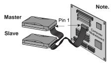
Note. If you are using a 40-pin 80-conductor cable, attach the *blue* connector to the motherboard, the *black* connector to the master drive, and the *grey* connector to the slave.
