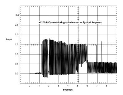
Figure 2. Typical 12V startup and operation current profile
