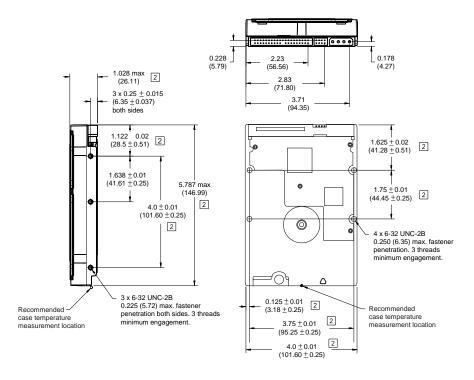
Figure 5. Mounting dimensions—top, side and end view
