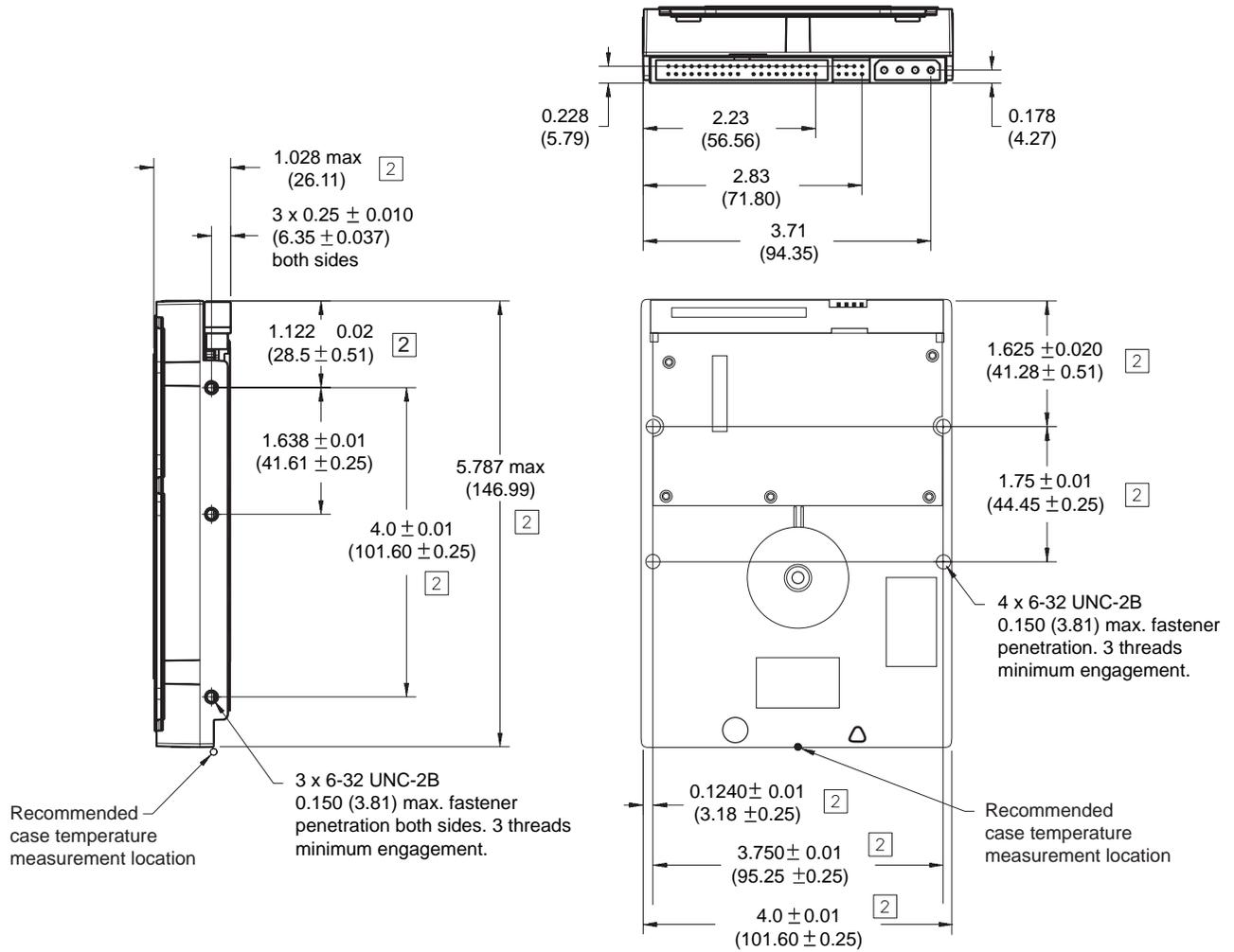
**Figure 6** Mounting dimensions—top, side and end view
