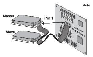
Note. If you are using a 40-pin, 80-conductor cable, attach the blue connector to the motherboard, the black connector to the master drive, and the gray connector to the slave.
