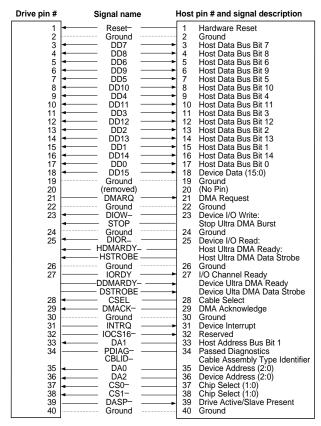
Pins 28, 34 and 39 are used for master-slave communication (details shown below).
