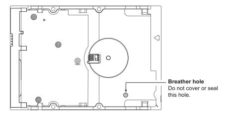
Figure 3 Breather filter hole location
