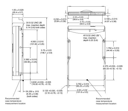
Figure 3. Mounting dimensions—top, side and end view
