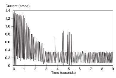
Figure 1. Typical startup and operation current profile
