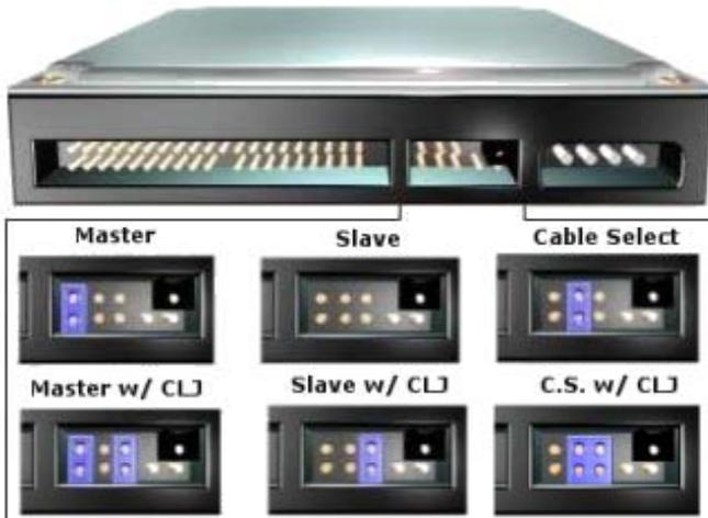
**(Master)** - A jumper placed over the DS pins configures the drive as a Master.
