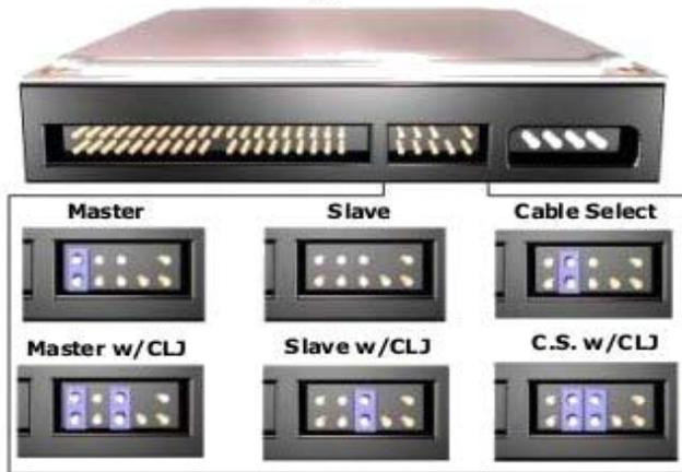
**(Master)** - A jumper placed over the DS pins configures the drive as a Master.
