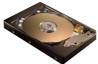
**Capacity****40GB****Model** ATA/133, 2MB buffer, FDB motor**2F040L0****Performance Specifications**
