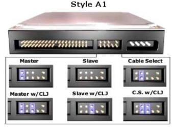
(Master) - The vertical jumper over the J50 pins is configuring the drive as a Master. The horizontal jumper over the J48 and J46 pins is in the Storage position.
