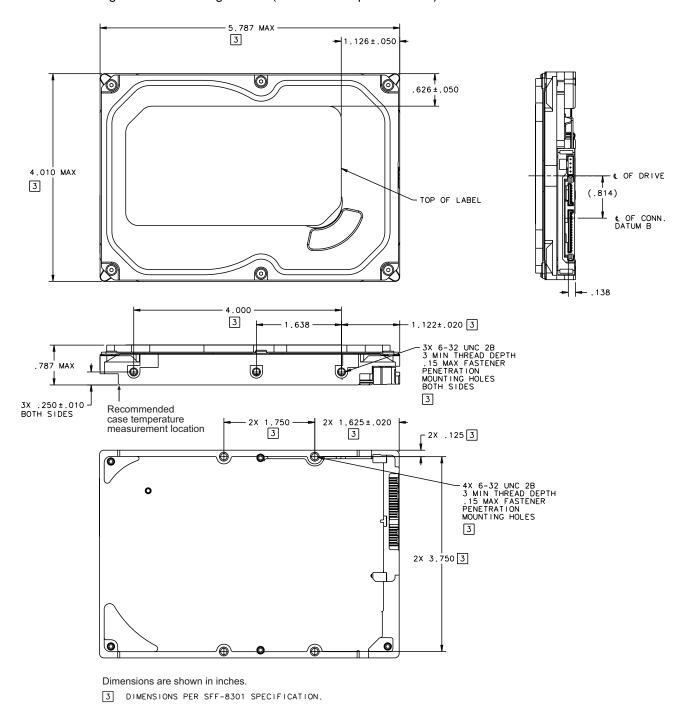
Figure 5. Mounting dimensions—top, side and end view
