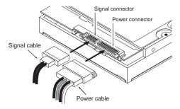
Figure 4. Attaching SATA cabling
