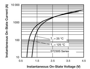
Fig. 7 - On-State Voltage Drop Characteristics
