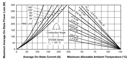
Fig. 3 - On-State Power Loss Characteristics
