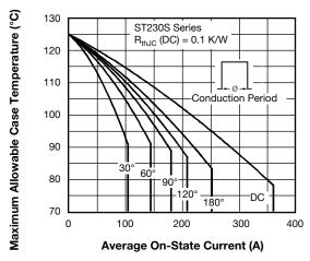
Fig. 2 - Current Ratings Characteristics
