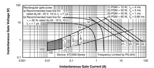
Fig. 9 - Gate Characteristics
