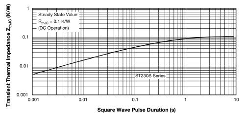
Fig. 8 - Thermal Impedance Z<sub>thJC</sub> Characteristics
