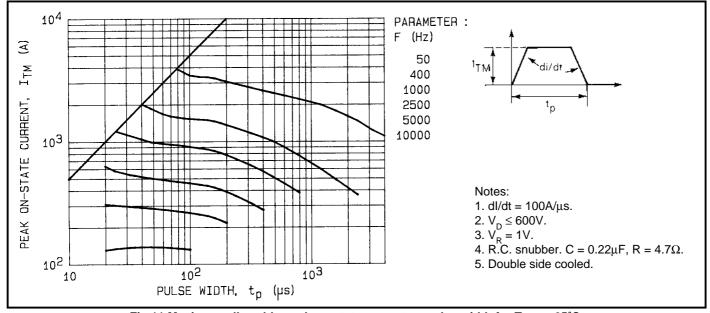
Fig.11 Maximum allowable peak on-state current vs pulse width for  $T_{case} = 65$  °C.
