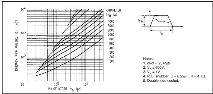
Fig.4 Energy per pulse for trapezoidal pulses
