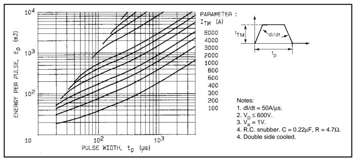
Fig.7 Energy per pulse for trapezoidal pulses.
