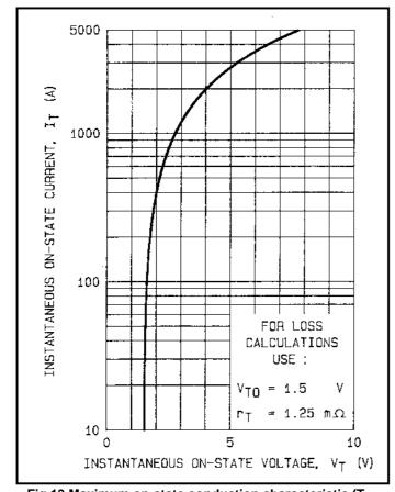
Fig.13 Maximum on-state conduction characteristic ( $T_j = 125^{\circ}C$ )
