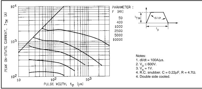
Fig.12 Maximum allowable peak on-state current vs pulse width for  $T_{case} = 90$ °C.
