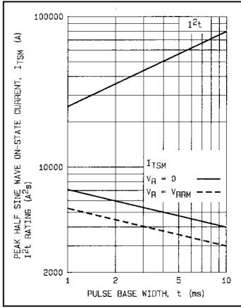
Fig.14 Non-repetitove sub-cycle surge on-state current and  $I^2$ t rating. (Initial  $T_j = 125$ °C)
