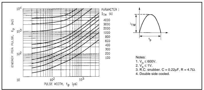
Fig.1 Energy per pulse for sinusoidal pulses.
