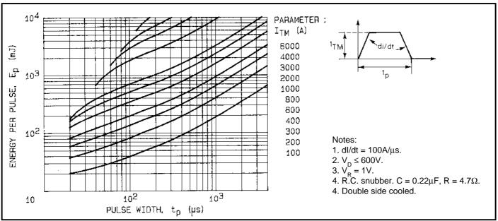
Fig.10 Energy per pulse for trapezoidal pulses.
