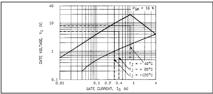
Fig.15 Gate trigger characteristics
