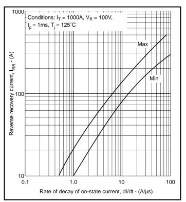
Fig.9 Reverse recovery current
