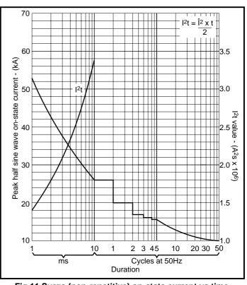
Fig.11 Surge (non-repetitive) on-state current vs time (with 50%  $V_{RRM}$  at  $T_{case} = 125$ °C)
