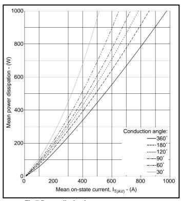
Fig.7 Power dissipation curves - square wave
