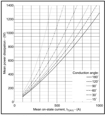
Fig.4 Power dissipation curves - sine wave
