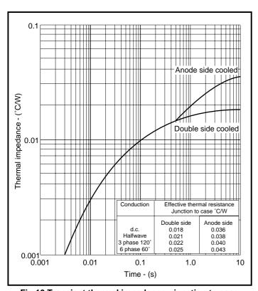
Fig.10 Transient thermal impedance - junction to case
