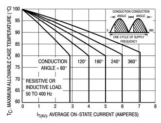
Figure 2. Current Derating (Full-Wave)
