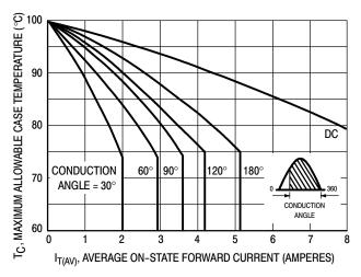
Figure 1. Current Derating (Half-Wave)
