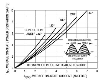
Figure 4. Maximum Power Dissipation (Full-Wave)
