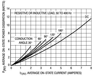
Figure 3. Maximum Power Dissipation (Half-Wave)
