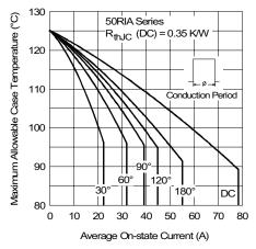
Fig. 2 - Current Ratings Characteristics
