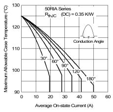
Fig. 1 - Current Ratings Characteristics
