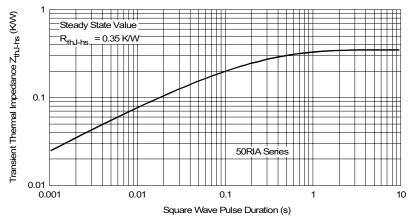
Fig. 8 - Thermal Impedance Z<sub>thJC</sub> Characteristics
