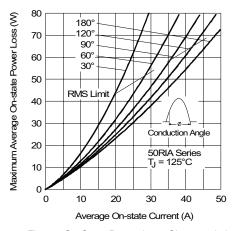
Fig. 3 - On-State Power Loss Characteristics
