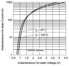
Fig. 7 - Forward Voltage Drop Characteristics
