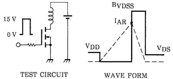
$T_{ch} = 25^\circ\text{C}$  (Initial)
