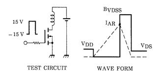
$$\begin{array}{l} T_{ch} = 25^{\circ}\!C~(Initial) \\ Peak~I_{AR} = 5~A,~R_G = 25~\Omega \end{array} ~E_{AS} = \frac{1}{2} \cdot L~\cdot I^2 \cdot ~(\frac{B_{VDSS}}{B_{VDSS} - V_{DD}}) \\ V_{DD} = 24~V,~L = 1.0~mH \end{array}$$
