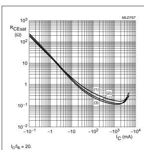
(1)  $T_{amb} = 150 \,^{\circ}\text{C}$ . (2)  $T_{amb} = 25 \,^{\circ}\text{C}$ . (3)  $T_{amb} = -55 \,^{\circ}\text{C}$ .
