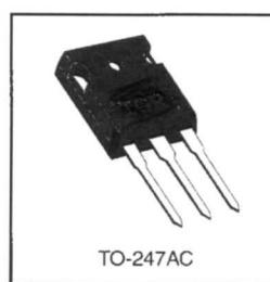
The TO-247 package is preferred for commercial-industrial applications where higher power levels preclude the use of TO-220 devices. The TO-247 is similar but superior to the earlier TO-218 package because of its isolated mounting hole. It also provides greater creepage distance between pins to meet the requirements of most safety specifications.
