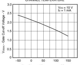
$T_{\text{ch}}$  - Channel Temperature -  $^{\circ}C$
