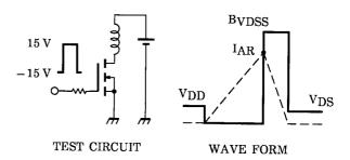
$$\begin{aligned} &RG = 25~\Omega \\ &V_{DD} = 90~V,~L = 1.79~mH \end{aligned} \qquad E_{AS} = \frac{1}{2} \cdot L \cdot I^2 \cdot \left( \frac{BV_{DSS}}{BV_{DSS} - V_{DD}} \right)$$
