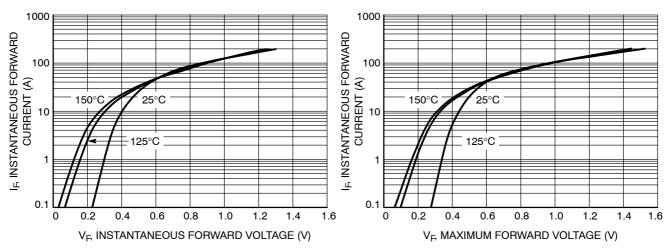
Figure 1. Typical Forward Voltage
