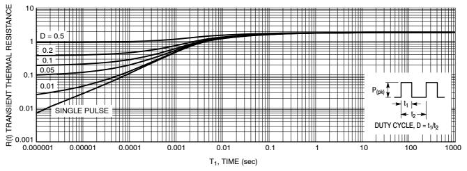
Figure 8. Thermal Response Junction-to-Case for MBR40L45CTG
