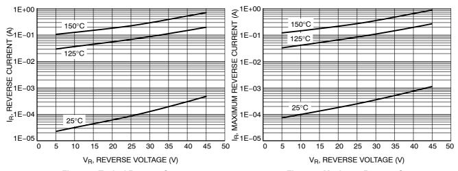
Figure 3. Typical Reverse Current
