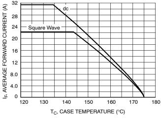
Figure 5. Current Derating, Case, Per Leg
