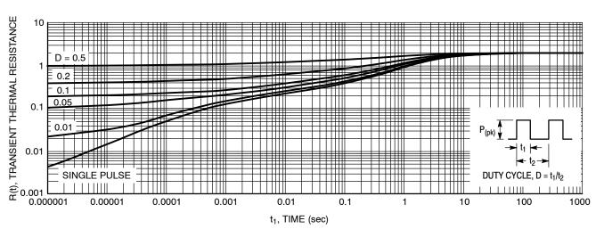
Figure 9. Thermal Response Junction-to-Case
