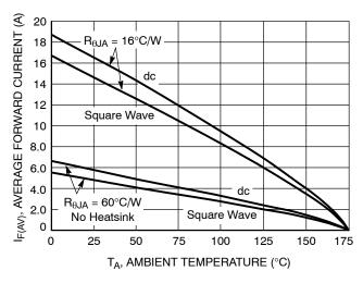
Figure 6. Current Derating, Ambient, Per Leg
