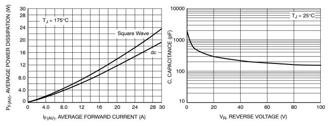
Figure 7. Forward Power Dissipation
