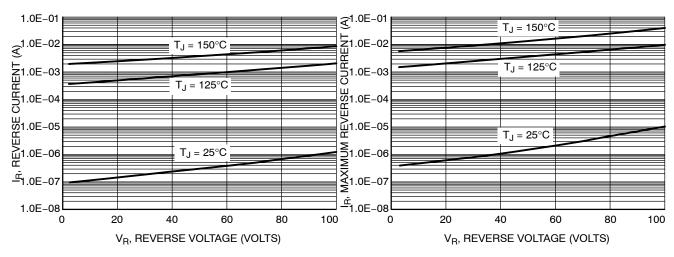
**Figure 3. Typical Reverse Current**
