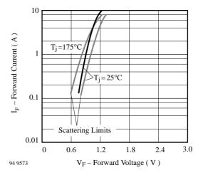
Figure 4. Forward Current vs. Forward Voltage
