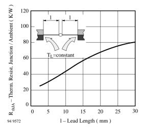
Figure 2. Thermal Resistance vs. Lead Length
