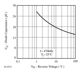
Figure 5. Diode Capacitance vs. Reverse Voltage
