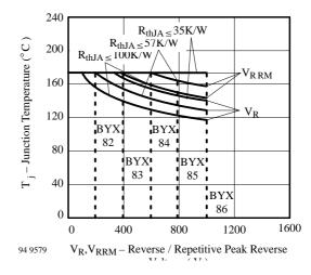
Figure 3. Junction Temperature vs. Reverse/Repetitive Peak Reverse Voltage
