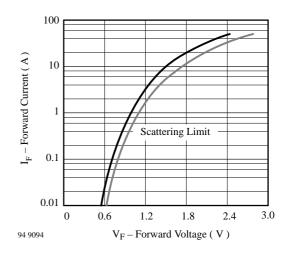
Figure 6. Forward Current vs. Forward Voltage
