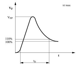
Figure 1. Turn on transient peak voltage
