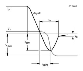
Figure 3. Turn off switching characteristic
