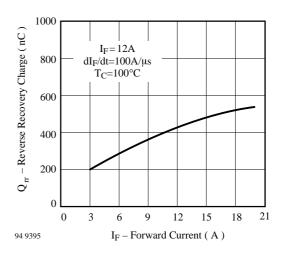
Figure 7. Reverse Recovery Charge vs. Forward Current
