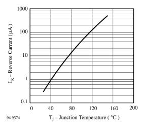
Figure 4. Reverse Current vs. Junction Temperature
