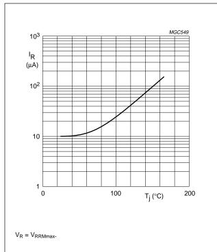
Fig.6 Reverse current as a function of junction temperature; maximum values.
