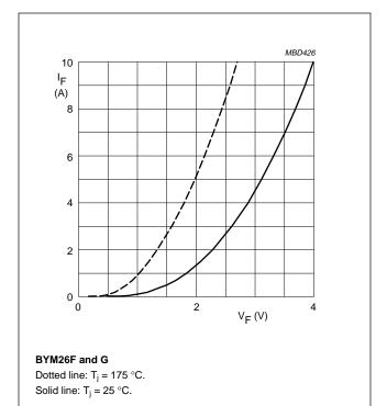
Fig.15 Forward current as a function of forward voltage; maximum values.
