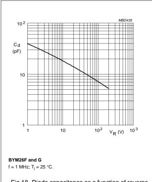
Fig.18 Diode capacitance as a function of reverse voltage; typical values.
