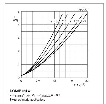
Fig.11 Maximum steady state power dissipation (forward plus leakage current losses, excluding switching losses) as a function of average forward current.
