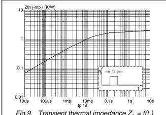
Fig.9. Transient thermal impedance  $Z_{th} = f(t_p)$
