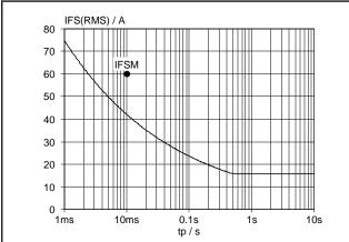
Fig.5. Maximum non-repetitive rms forward current.  $I_F = f(t_p)$ ; sinusoidal current waveform;  $T_j = 150$ °C prior to surge with reapplied  $V_{RWM}$ .
