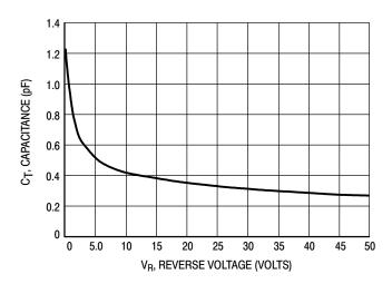
Figure 3. Typical Capacitance
