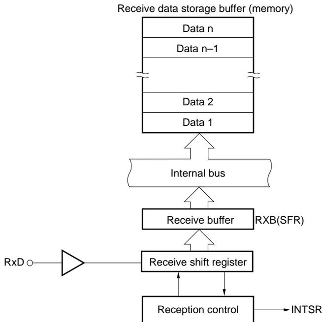
Each time macro service request (INTSR) is generated, the receive data is transferred from RXB to memory. When data n (last byte) has been transferred to memory (when the receive data storage buffer has become full), vectored interrupt request (INTSR) is generated.
