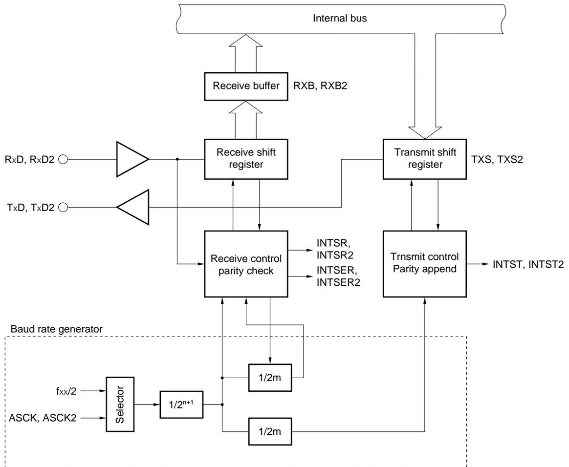
**Remark**  $f_{xx}$ : oscillation frequency or external clock input
