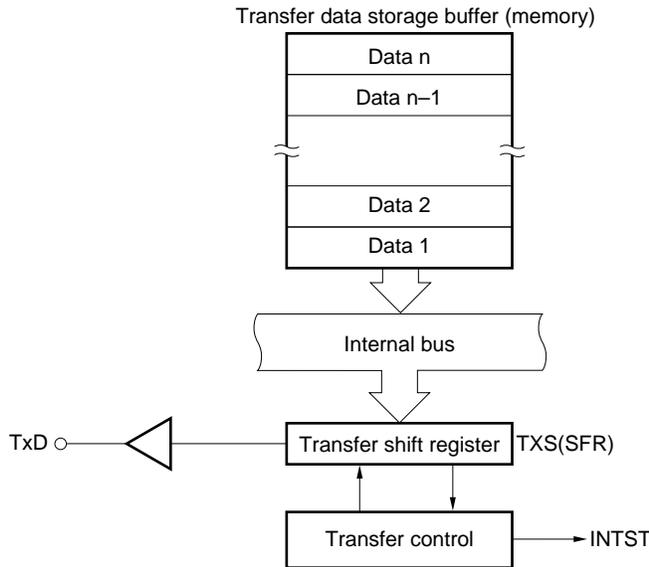
Each time macro service request (INTST) is generated, the next transfer data is transferred from memory to TXS. When data n (last byte) has been transferred to TXS (when the transfer data storage buffer has become empty), vectored interrupt request (INTST) is generated.
