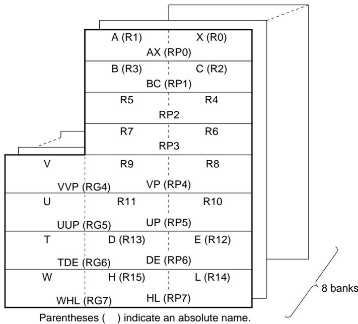
**Caution** Registers R4, R5, R6, R7, RP2, and RP3 can be used as X, A, C, B, AX, and BC registers, respectively, by setting the RSS bit of the PSW to 1. However, use this function only for recycling the program of the 78K/III Series.
