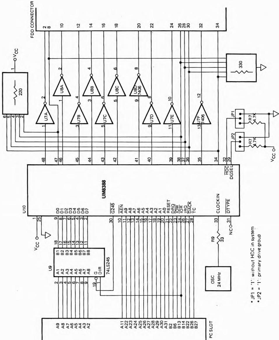
**Figure A-1 PC/AT (1.44M, 1.2M, 720K, 360K FDD) Application Circuit**
