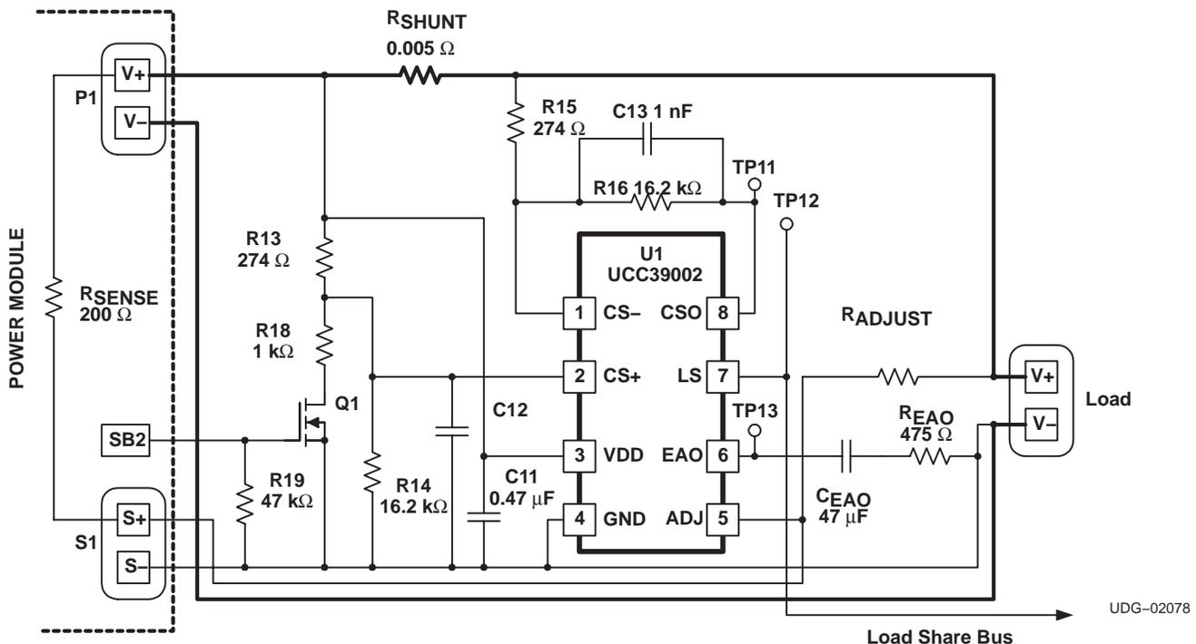
**Figure 5. Typical High-Side Application for Single Power Module**
