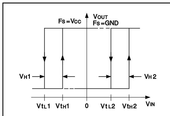
Figure 1.  $V_{tL}$ ,  $V_{tH}$ ,  $V_H$  Definition
