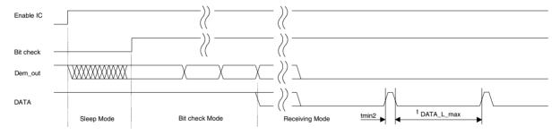
After the end of a data transmission, the receiver remains active and random noise pulses appear at pin DATA. The edge-to-edge time period  $t_{ee}$  of the majority of these noise pulses is equal to or slightly higher than  $T_{DATA\ min}$ .
