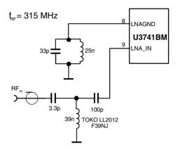
Please note that for all coupling conditions (see Figure 3 and Figure 4), the bond wire inductivity of the LNA ground is compensated. C3 forms a series resonance circuit together with the bond wire. L = 25 nH is a feed inductor to establish a DC path. Its value is not critical but must be large enough not to detune the series resonance circuit. For cost reduction, this inductor can be easily printed on the PCB. This configuration improves the sensitivity of the receiver by about 1 dB to 2 dB.
