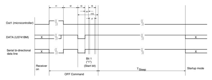
Figure 18. Timing Diagram of the OFF Command Via Pin ENABLE
