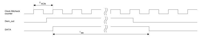
Figure 15. Debouncing of the Demodulator Output
