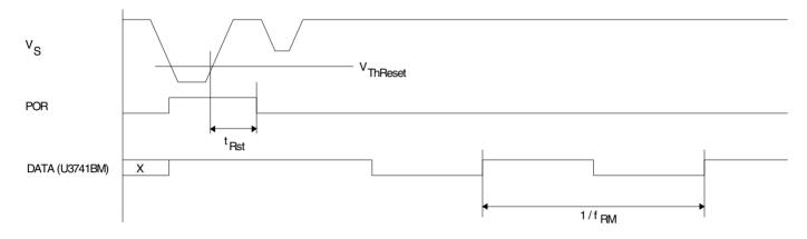
Figure 20. Timing of the Register Programming
