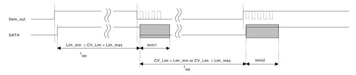
Figure 16. Steady L State Limited DATA Output Pattern after Transmission
