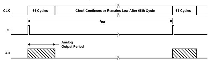
**Figure 1. Timing Waveforms**
