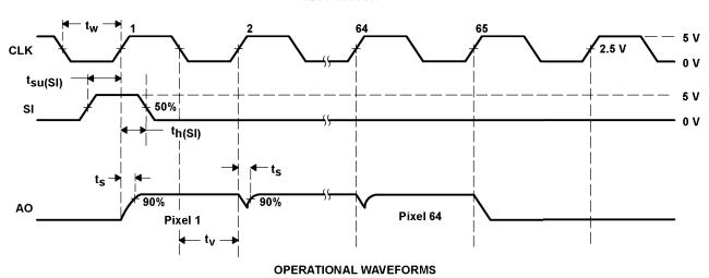
Figure 2. Test Circuit and Operational Waveforms
