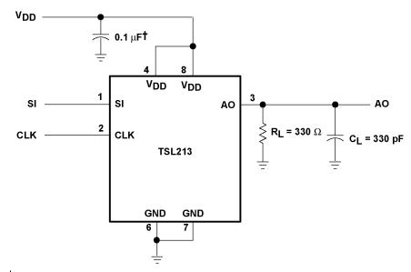
† Supply bypass capacitor with short leads should be placed as close to the device as possible.
