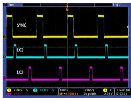
Figure 32. Synchronization at 500 kHz
