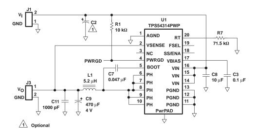
Figure 10. TPS54314 Schematic
