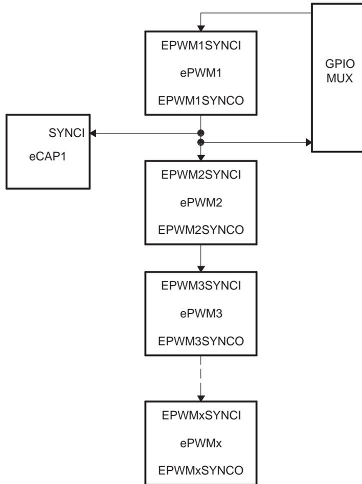
Scheme 2 shown in [Figure 8](#) is used by the 2804x devices when the ePWM pinout is configured for A-channel only mode (GPAMCFG[EPWMMODE] = 3). If the 2804x ePWM pinout is configured for 280x compatible mode (GPAMCFG[EPWMMODE] = 0), then Scheme 1 is used.
