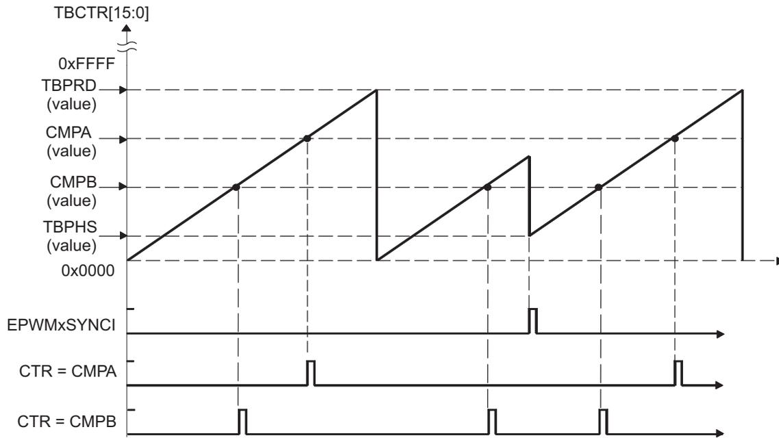
NOTE: An EPWMxSYNCl external synchronization event can cause a discontinuity in the TBCTR count sequence. This can lead to a compare event being skipped. This skipping is considered normal operation and must be taken into account.
