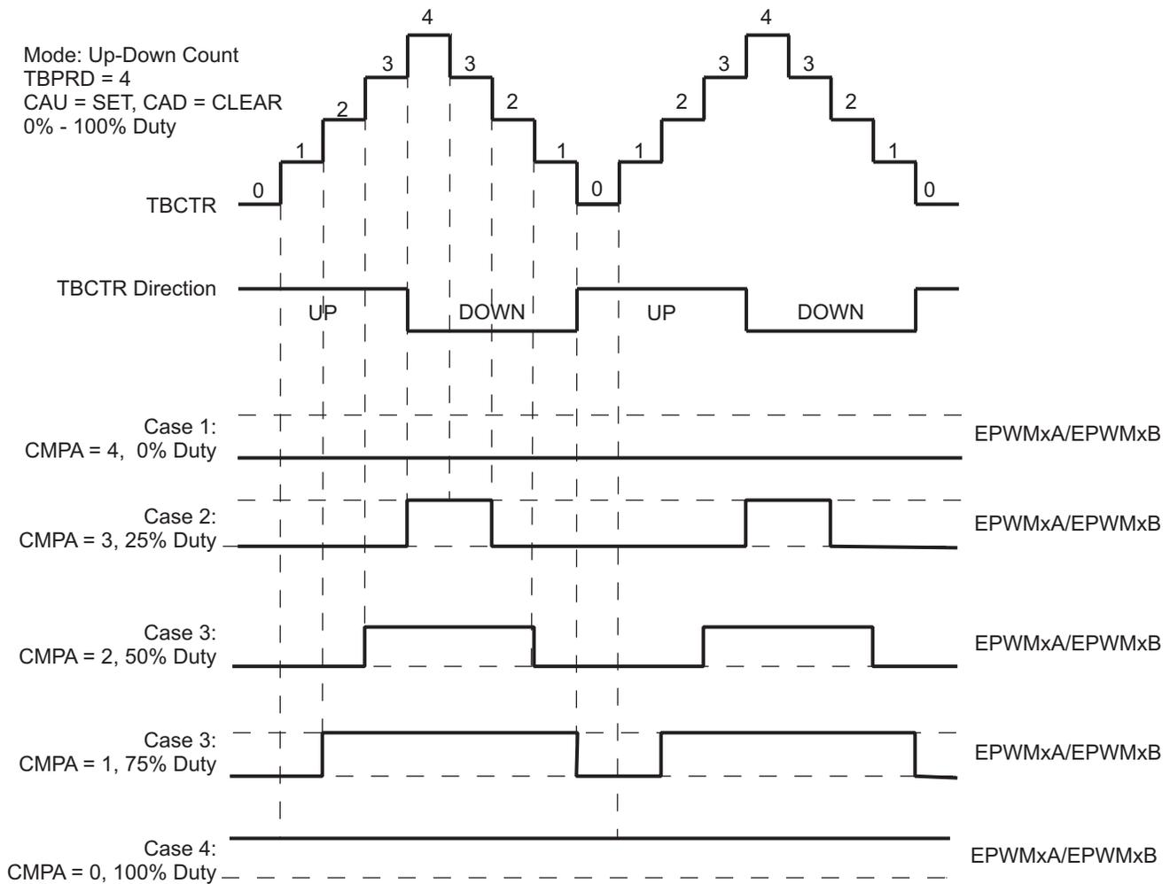
The PWM waveforms in [Figure 24](#) through [Figure 29](#) show some common action-qualifier configurations. The C-code samples in [Example 1](#) through [Example 6](#) shows how to configure an ePWM module for each case. Some conventions used in the figures and examples are as follows:
