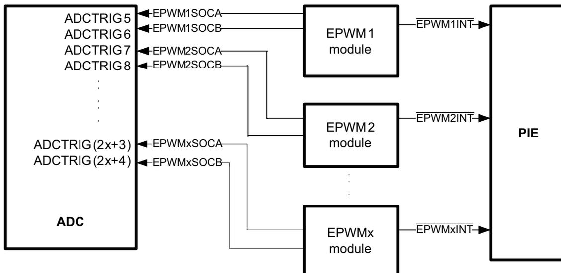
The event-trigger submodule monitors various event conditions (the left side inputs to event-trigger submodule shown in Figure 43) and can be configured to prescale these events before issuing an Interrupt request or an ADC start of conversion. The event-trigger prescaling logic can issue Interrupt requests and ADC start of conversion at:
