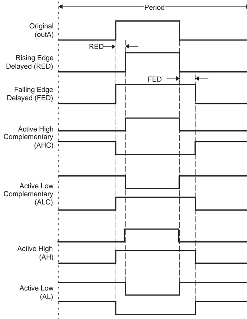
The dead-band submodule supports independent values for rising-edge (RED) and falling-edge (FED) delays. The amount of delay is programmed using the DBRED and DBFED registers. These are 10-bit registers and their value represents the number of time-base clock, TBCLK, periods a signal edge is delayed by. For example, the formula to calculate falling-edge-delay and rising-edge-delay are:
