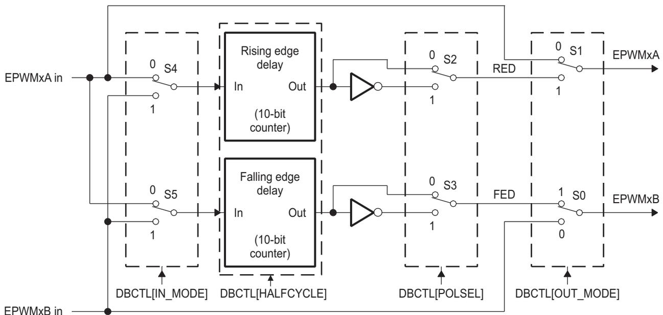
Although all combinations are supported, not all are typical usage modes. [Table 14](#) documents some classical dead-band configurations. These modes assume that the DBCTL[IN\_MODE] is configured such that EPWMxA In is the source for both falling-edge and rising-edge delay. Enhanced, or non-traditional modes can be achieved by changing the input signal source. The modes shown in [Table 14](#) fall into the following categories:
