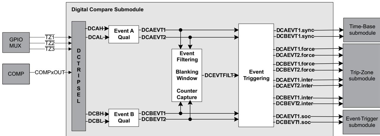
The digital compare (DC) submodule compares signals external to the ePWM module (for instance, COMPxOUT signals from the analog comparators) to directly generate PWM events/actions which then feed to the event-trigger, trip-zone, and time-base submodules. Additionally, blanking window functionality is supported to filter noise or unwanted pulses from the DC event signals.
