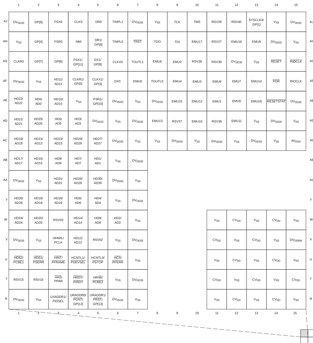
Figure 2-2. C6455 Pin Map (Bottom View) [Quadrant A]
