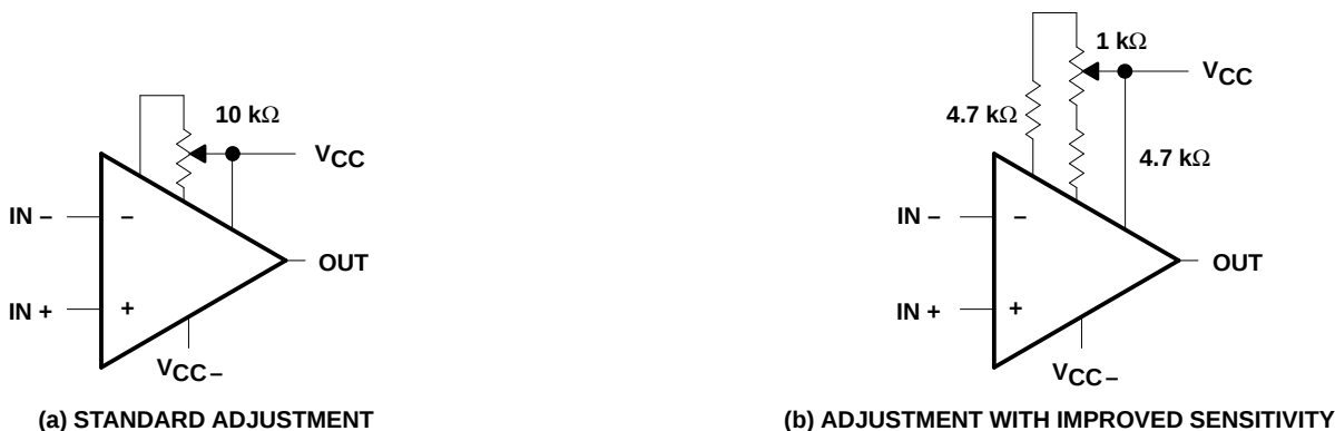
Figure 47. Input Offset-Voltage Nulling Circuits
