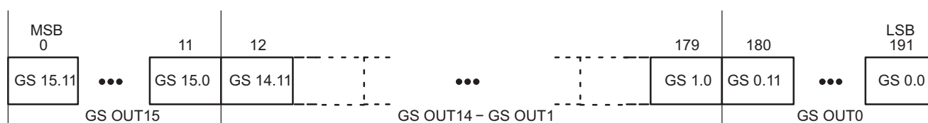
Figure 17. Grayscale Data Packet Format
