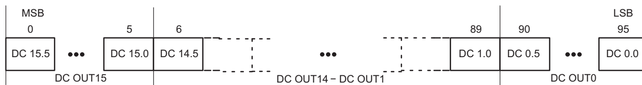
Figure 15. Dot Correction Data Packet Format
