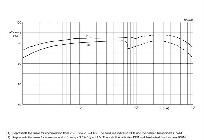
Fig.5 Efficiency as a function of load current I<sub>L</sub>.
