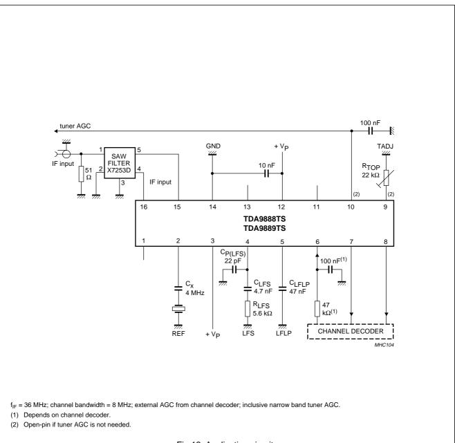
Fig.12 Application circuit.
