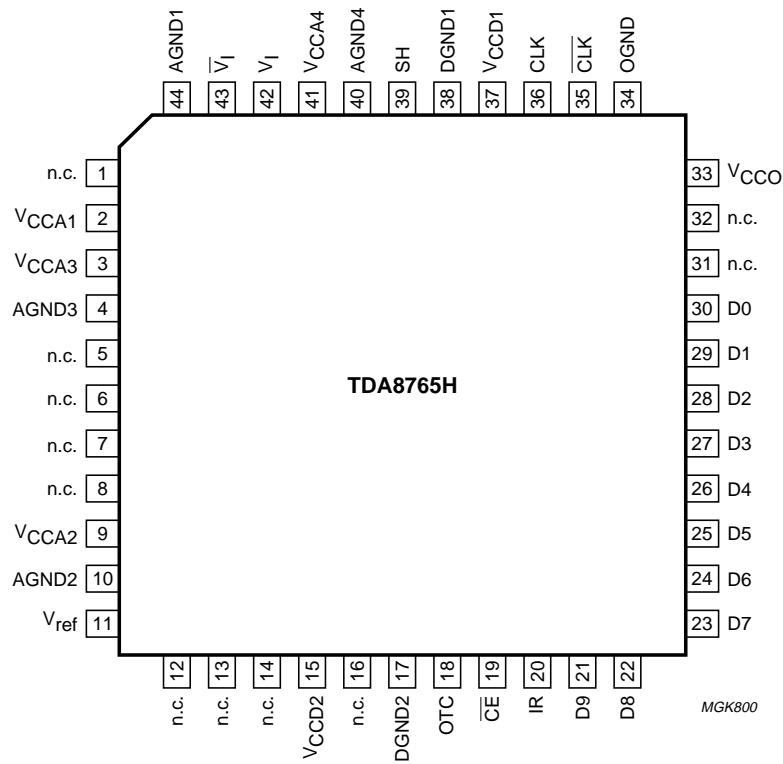
Fig.2 Pin configuration.
