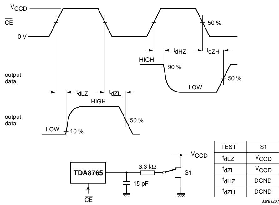
Fig.6 Timing diagram and test conditions of 3-state output delay time.
