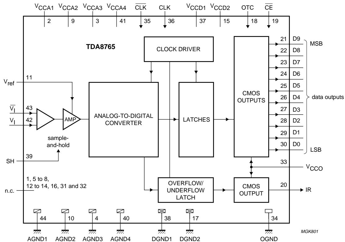
Fig.1 Block diagram.
