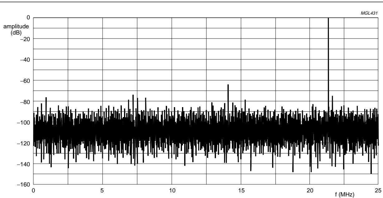
Fig.4 Typical fast Fourier transform ( $f_{CLK} = 50$  MHz;  $f_i = 21.4$  MHz).
