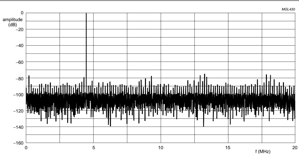
Fig.3 Typical fast Fourier transform ( $f_{CLK} = 40$  MHz;  $f_i = 4.43$  MHz).
