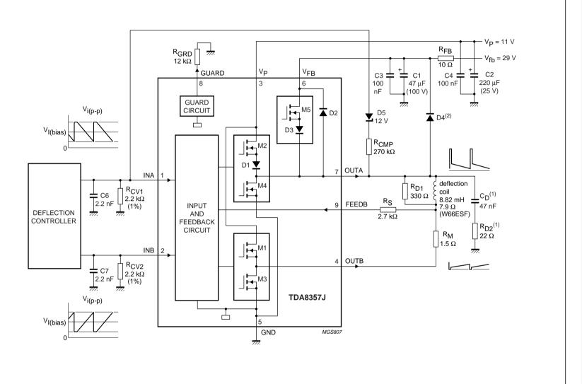
$f_{vert} = 50 \text{ Hz}$ ;  $t_{FB} = 640 \mu s$ ;  $I_{I(bias)} = 400 \mu A$ ;  $I_{i(dif)(peak)} = 494 \mu A$ ;  $I_{O(p-p)} = 1.45 A$ .
