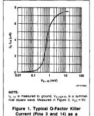
Function of the Peak-to-Peak Input Voltage (V<sub>2</sub>-15)
